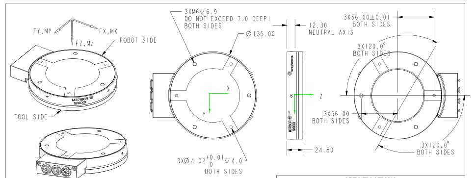
POSITIVE OUTPUT WHEN THE LOAD IS APPLIED TO THE TOOL SIDE PER COORDINATE SYSTEM AS SHOWN
